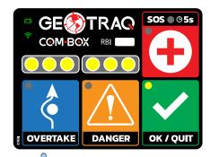
Vehicle A wants to overtake vehicle B: press for 2 seconds, the BLUE BUTTON, to send a signal to the vehicle B ahead (must be less than 200m ahead).
