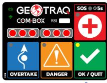
If you receive a SOS signal from another vehicle, your lights will BLINK RED. ALARM IS ON. **CONFIRM WITH OK/QUIT BUTTON, ALARM WILL** STOP. Lights will continue BLINKING RED FOR **30 SECONDS.** BE READY TO ASSIST AN ACCIDENT SCENE.
